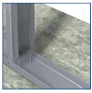
Place 24" Midwall against stud web. Placebase plate to anchors through pre-drilled guide holes.
